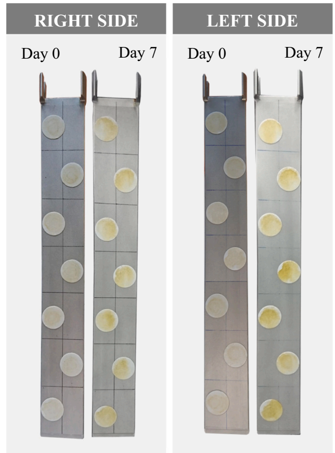
Fig. 7. Photographic comparison of biofilm disks inoculated on the left side and right side of the PSBR support panel on the day of launch (Day 0) and after harvest (Day 7).
